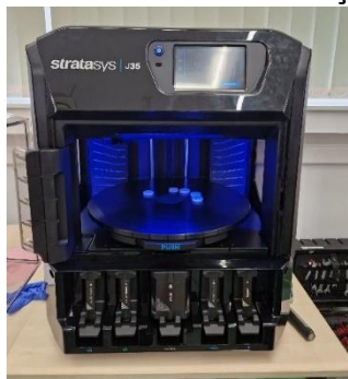
Imprimanta 3D - Stratasys J35 Pro, Polyjet
