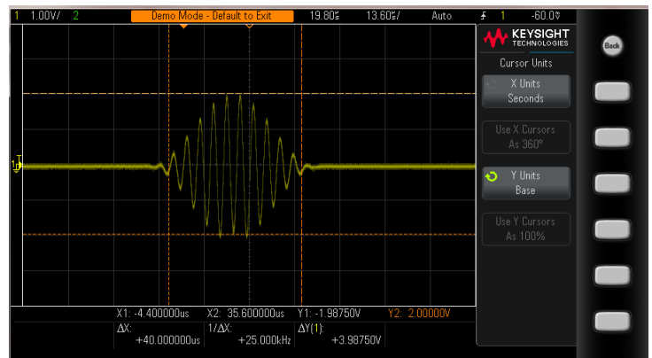
Figure 3: Cursors allow quick and accurate measurements, here measuring the RF burst of 40 usec, and 4 Volts.
