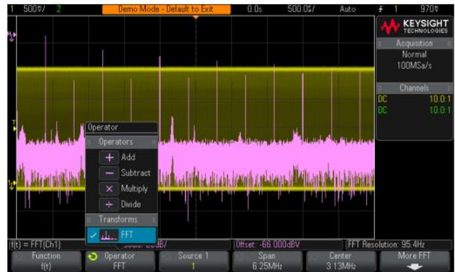
Figure 6: Define the exact FFT required with simple controls to set the analysis bandwidth.
