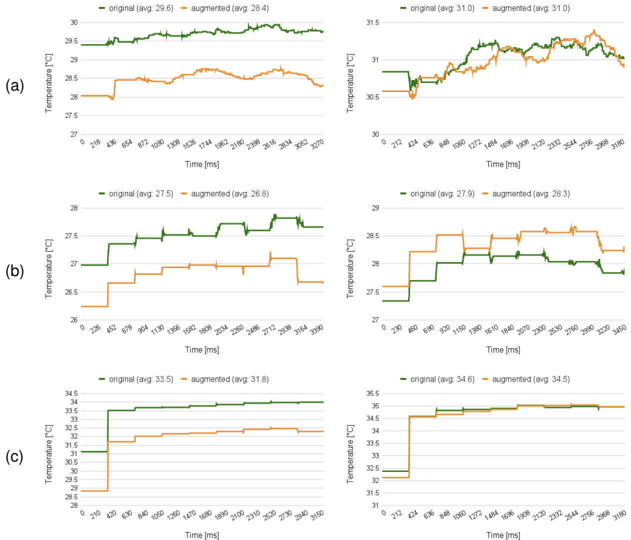
Figure 34: Results with mathematical computations as a noise, selecting CPU affinity, a) contains the results for ls and chmod commands for system D-150a , b) contains results for D-151a and c) for D-152a .
