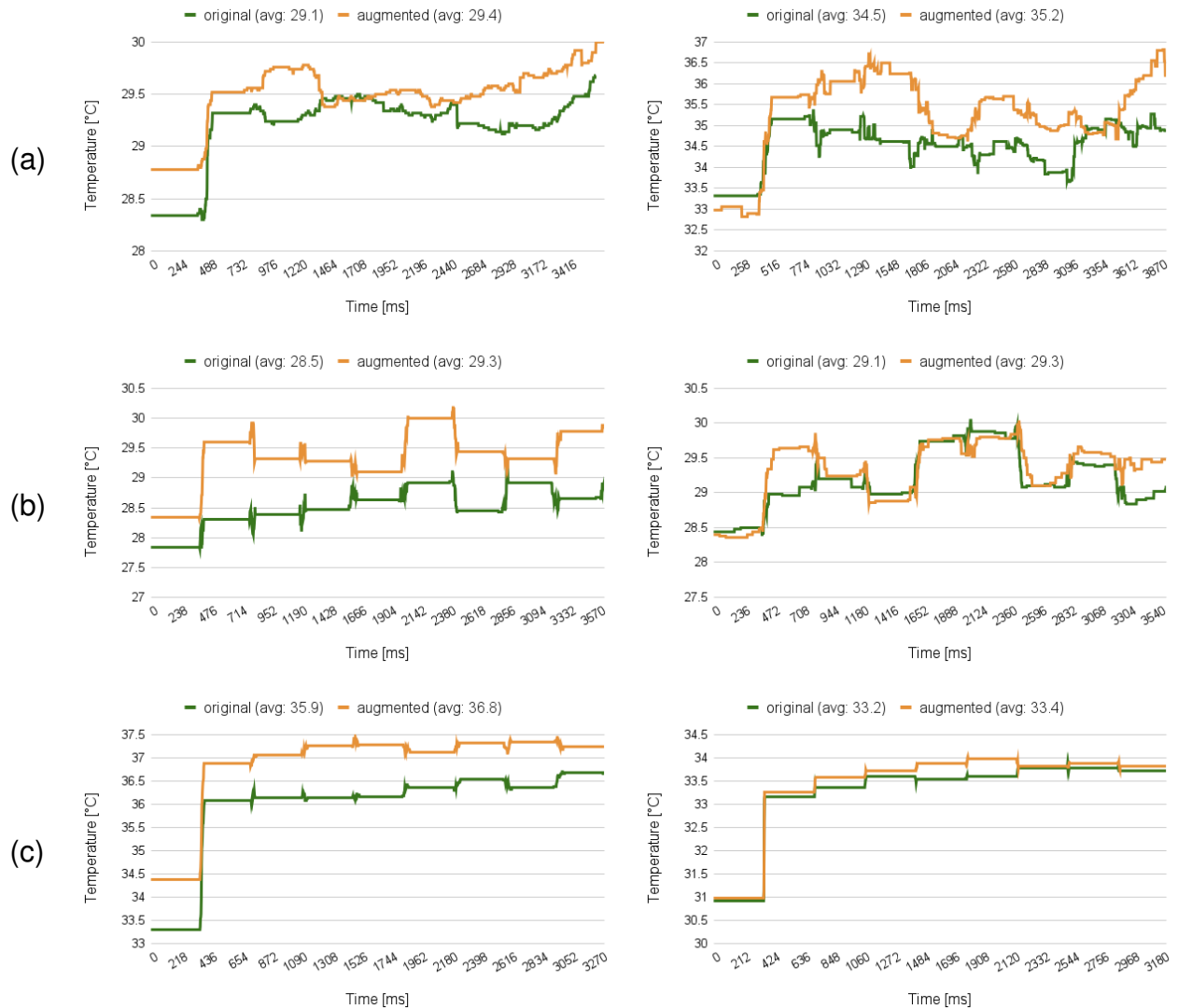
Figure 32: Results with surfing the browser as a noise, selecting CPU affinity, a) contains the results for ls and chmod commands for system D-150a , b) contains results for D-151a and c) for D-152a .
